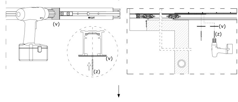
Using the Rear Adjustable Stop Bar Screws (U) provided, attach the metal bar to the top track to lock the rear adjustable stop into place. Ensure these screws are flush to the stop bar and not at an angle else the head of the screw can catch on the components inside the track.
