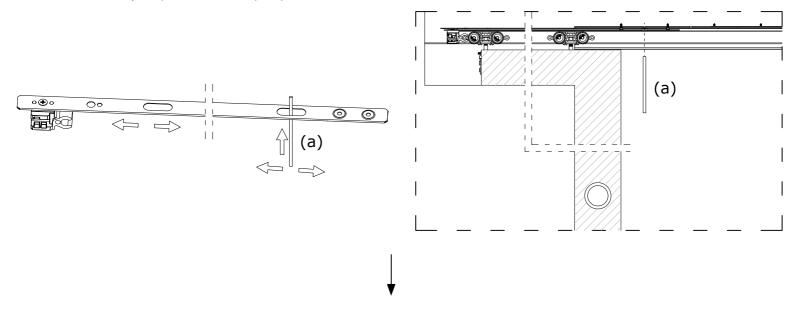
Using the Drilling Guide (V) and the Drill Bit (Z) provided, drill holes into the top of the Aluminium track through the fixing holes in the metal bar. Ensure these holes are drilled straight.
